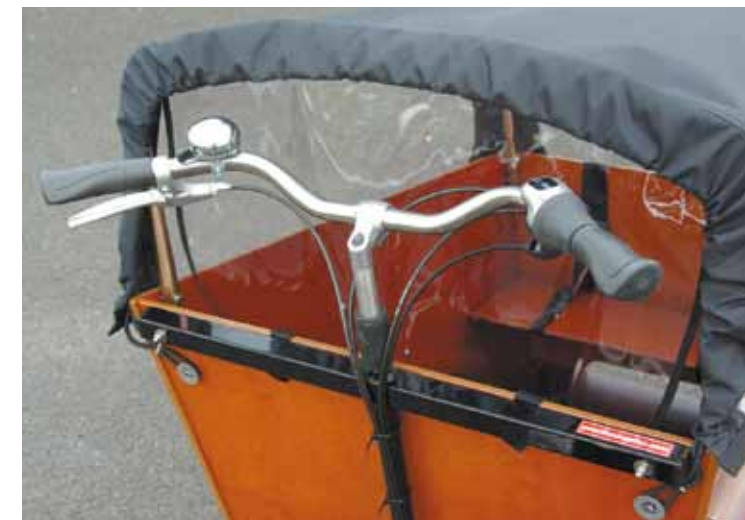
ABOVE: Wide, swept-back bars fixed to the load box provide plenty of leverage to steer the Bakfiets.
