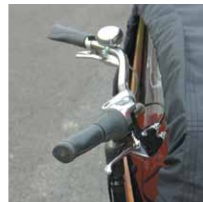
ABOVE: Wide, swept-back bars fixed to the load box provide plenty of leverage to steer the Bakfiets.
